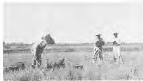
Geologists using a resistivity machine during an aquifer study.
