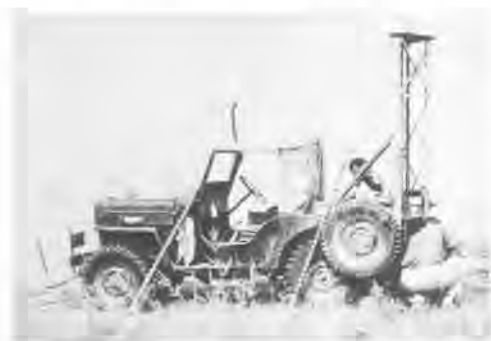
Jeep-mounted auger rig used for test drilling during mapping of a geologic quadrangle.
