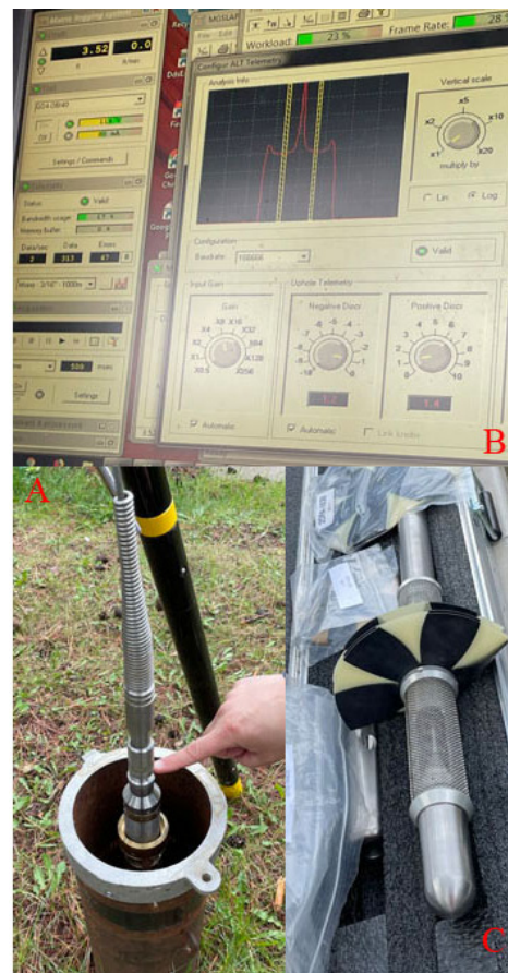
Figure 3. New Borehole geophysical equipment: (a) setting starting depth for logging; (b) software interface within the logging van; (c) heat pulse flowmeter.
