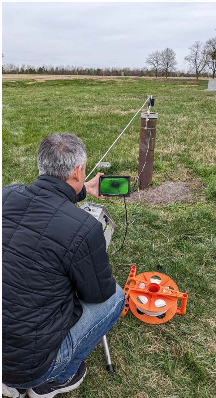
Figure 2. DGS hydrogeologist inspecting a monitoring well using a down-well video camera.
