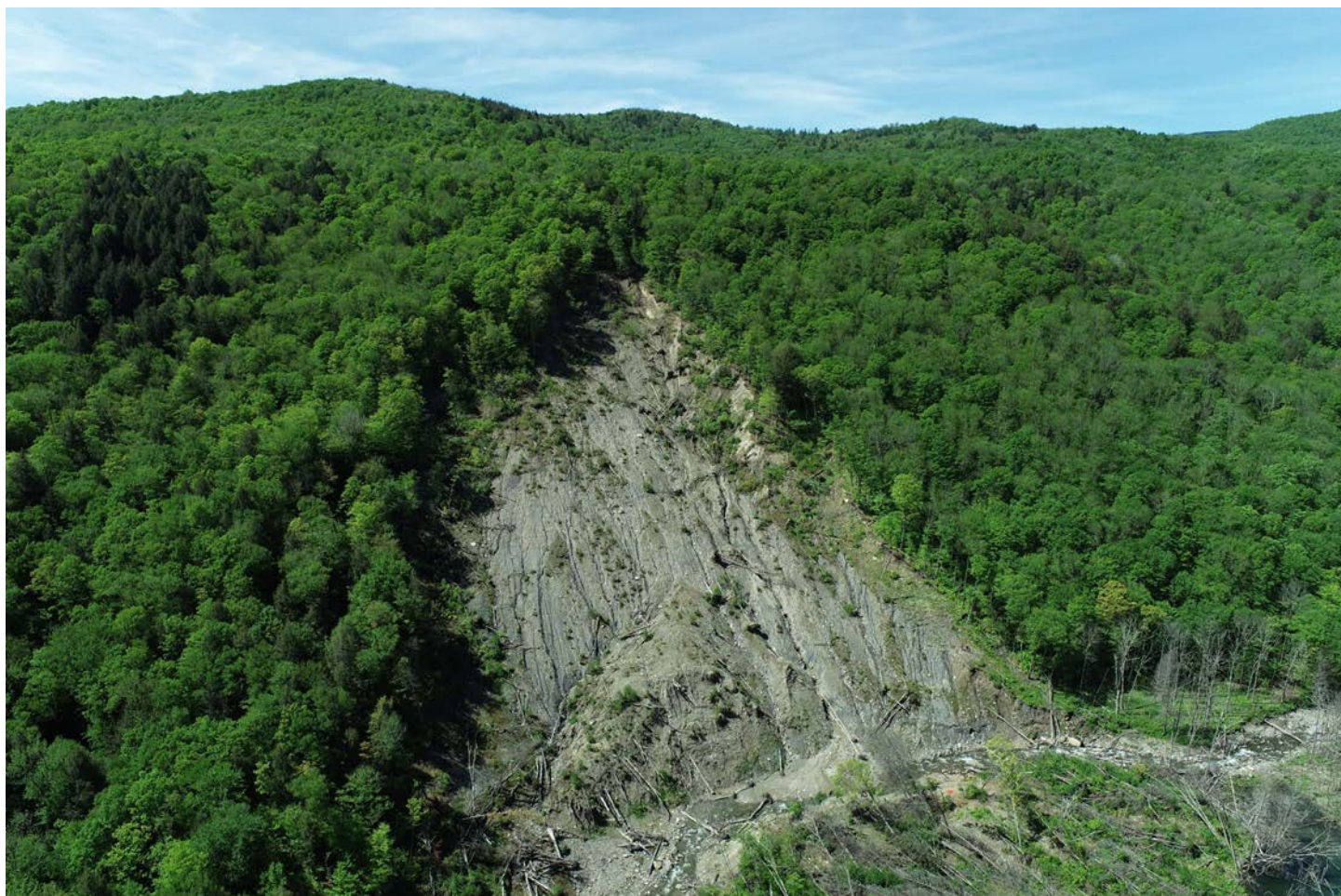
Figure 1. Oblique view of the 12+ acre Cotton Brook landslide that was triggered in 2019. A portion of the toe deposit is shown across the river in the bottom of the view; the dead standing trees in the lower right were submerged under water for several weeks when the Little River was dammed by the toe deposit.
