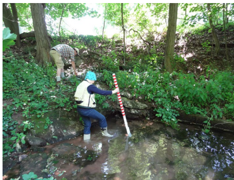
Figure 1. BTGS geologists measuring the discharge at Derry Spring, Dauphin County, Pennsylvania. Flow from the limestone spring was estimated at 519 gallons per minute. (June 2016)
