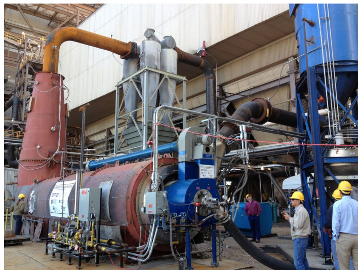
Figure 5. Full-scale demonstration testing of the SAP technology for flue gas mercury removal at a 650-MWe power plant.
