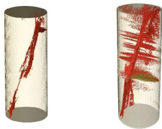
Figure 1. Reconstruction from micro-CT scans of a Castlegate outcrop plug (left) and a Mt. Simon Sandstone core plug (right), after testing in a triaxial load frame. During testing, a weak fracture plane was created by increasing differential applied stress past the shear
