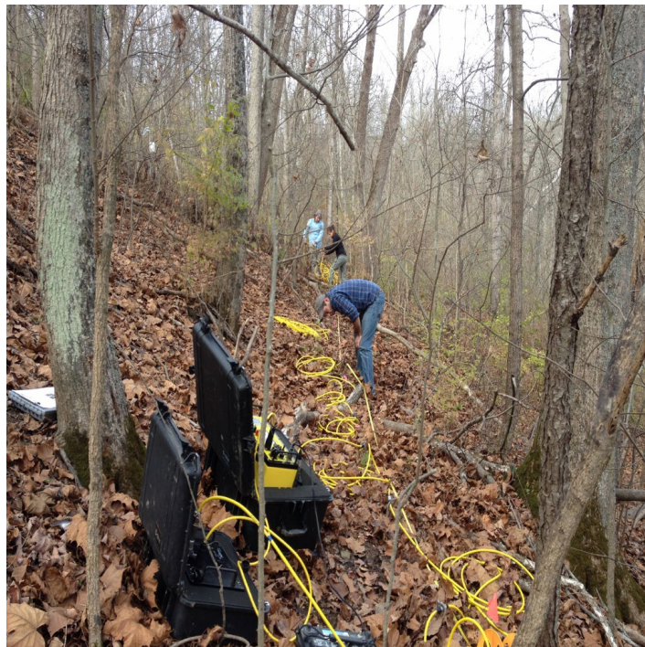
Figure 2. KGS students and staff conduct an electrical resistivity survey for landslide characterization at a site in northern Kentucky.
