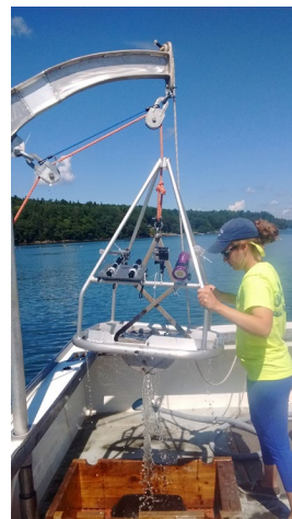
Figure 9. Benthic grab sampling near the mouth of the Kennebec River provides ground truth for sediment types imaged by the multibeam sonar system.
